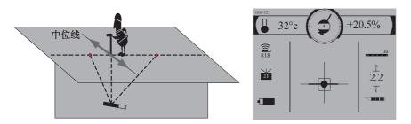
Warning: GL600 locating system uses the transmitter's magnetic field to locate the transmitter. It prefers smooth movements rather than sudden changes of direction.
